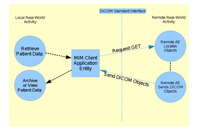
After performing a C-FIND operation, either the user (using the MIM Client Application) or an automated process (in the MIM Assistant) initiates a retrieval operation. The MIM AE sends a C-GET request for the data in question. The remote AE locates the objects in question, and then sends the requested objects on the same association. The DICOM objects are then shown on screen or archived to make them available for further processing.
