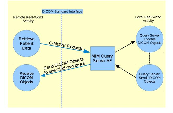
A remote AE initiates a retrieval operation for a specified set of DICOM objects, using a C-MOVE request specifying to which remote AE the data should be sent. The MIM Query Server AE locates the objects in question, and then initiates a new association to the specified remote AE either on the requesting machine or a different machine. The DICOM objects are then sent via C-STORE to the remote AE, which archives them or processes them in some other fashion.
