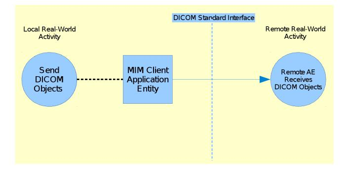
The MIM Client AE or MIM Assistant AE sends DICOM objects to a remote AE. This activity is initiated either by user action in the MIM Client application or by an automated process in the MIM Assistant service.
