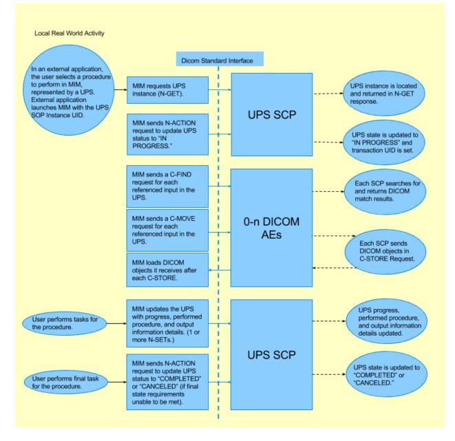
The user browses UPS work items listed in an external application and chooses a work item to be performed in MIM. The external application launches the MIM application using its CLI to identify the UPS representing the work item to be performed. The MIM AE takes ownership of the UPS on the UPS SCP and automatically walks the user through performing the procedure, informing the UPS SCP about progress updates, and completion/cancellation.
