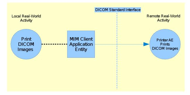
A user initiates a DICOM Print operation in the MIM Client Application. The MIM AE creates a print job on the Printer AE and instructs it to print the specified DICOM images.
