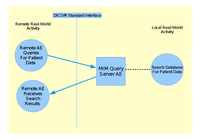
A remote AE queries the MIM Query Server AE for patient data. The MIM Query Server AE searches its database and returns the search results to the remote AE.
