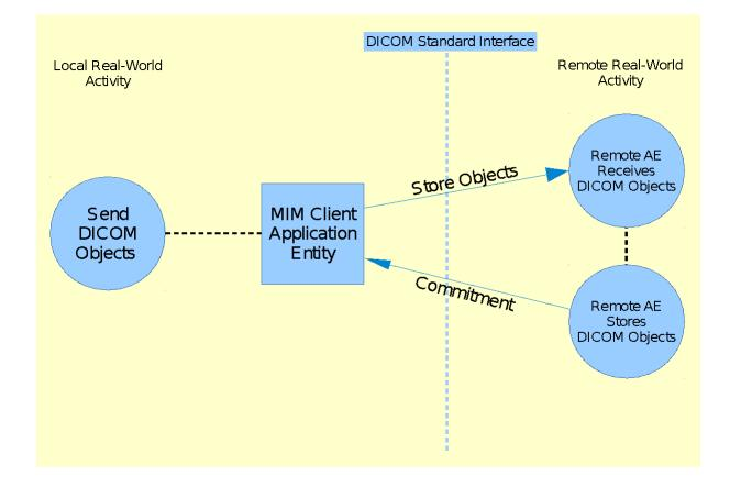
The MIM Client AE or MIM Assistant AE sends DICOM objects to a remote AE that is configured to use Storage Commitment. This activity is initiated either by user action in the MIM Client application or by an automated process in the MIM Assistant service.
